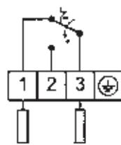
Switching and interlocking with rising pressure. Additional function ZF205.
