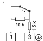
Normally closed contact **with reclosing lockout** and resistor combination, for **maximum pressure monitoring**, plastic-coated housing (chemical version).
