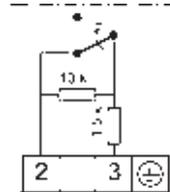
Normally closed contact **with reclosing lockout** and resistor combination, for **minimum pressure monitoring**, plastic coated housing (chemical version).
