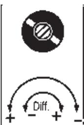
With pressure switches from the DWAMV and DWR...-203 series, the direction of action of the differential screw is reversed.
