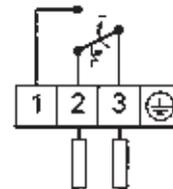
Switching and interlocking with falling pressure. Additional function ZF206.
